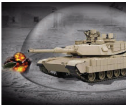
The Trophy vetronics system will protect U.S. main battle tanks from rocket-propelled grenades, anti-tank guided missiles, and similar anti-armor threats.
