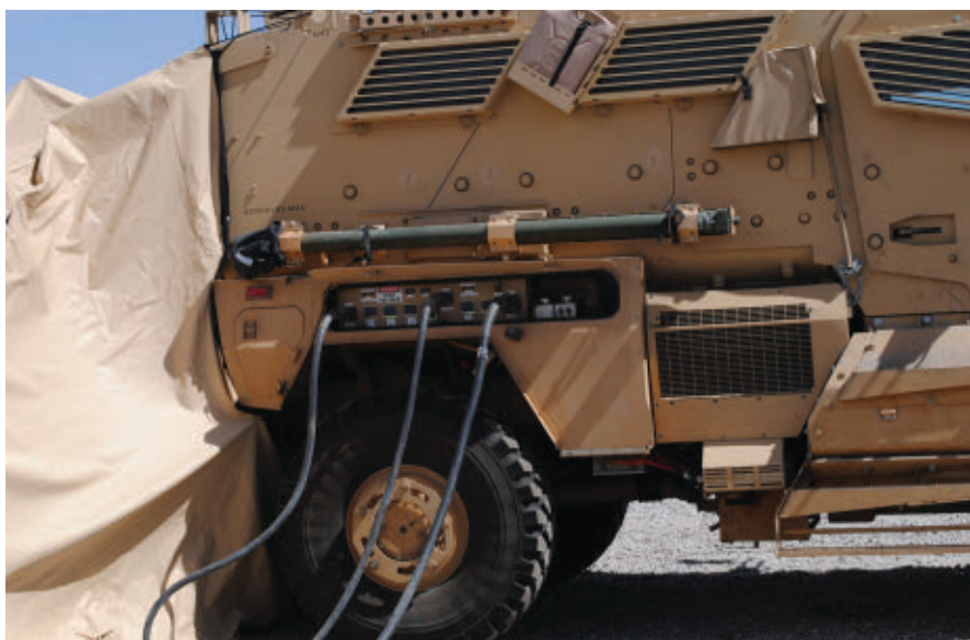
The Leonardo DRS TITAN On Board Vehicle Power (OBVP) system uses a transmission integral generator is able to produce as much vehicle power as 125 kilowatts.
