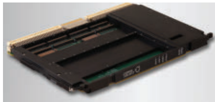
The Curtiss-Wright VME-1910 features Intel's 6-core hyper-threading Intel 8th Gen "Coffee Lake" E-2176M Xeon processor with integrated graphics and supports today's latest software and security advances.
