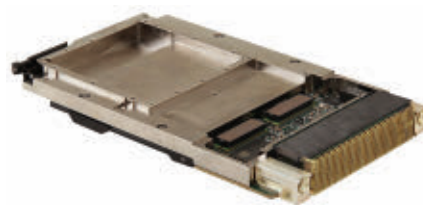
The Curtiss-Wright CHAMP-XD1S high-performance 3U OpenVPX digital signal processor (DSP) engine is a multi-core High Performance Embedded Computing (HPEC) module with advanced security features.
