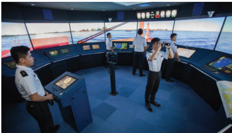
Ocean-going ship bridges are large and complex. To train bridge crews, simulators must equal their size and complexity, as demonstrated by this bridge crew simulator at the Philippines' United Marine Training Center.
