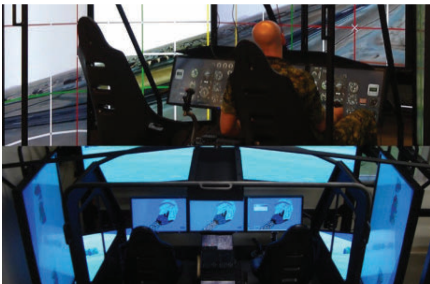
This photo shows a simulation and mission rehearsal system for the Bell CH-146 Griffon multi-role utility helicopter, a variant of the Bell 412EP for the Canadian Armed Forces.
