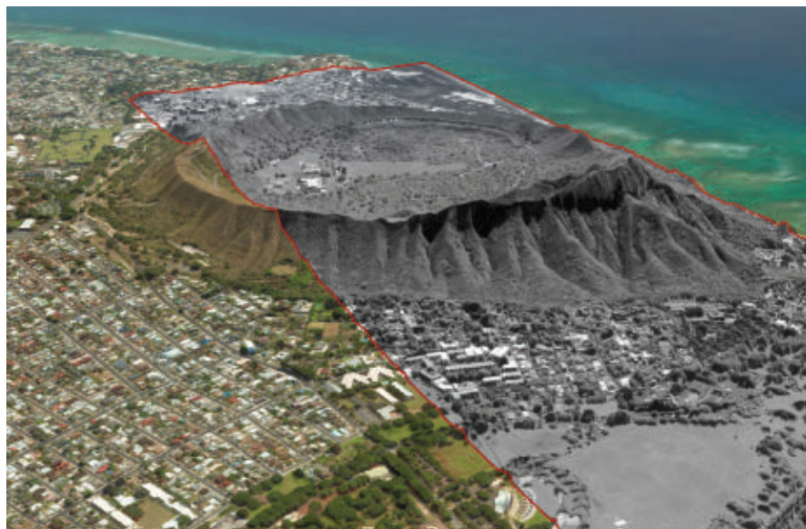
The Vricon Precision 3D Registration (P3DR) georegisters sensor data with a 3D model in real time to measure coordinates without the need for ground-control points.
