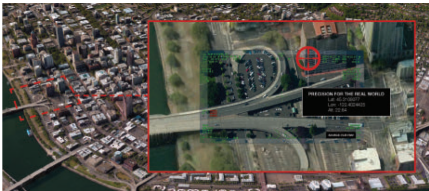
The Vicon P3DR can georegister full-motion video, providing accurate coordinates, even on the sides of buildings.
