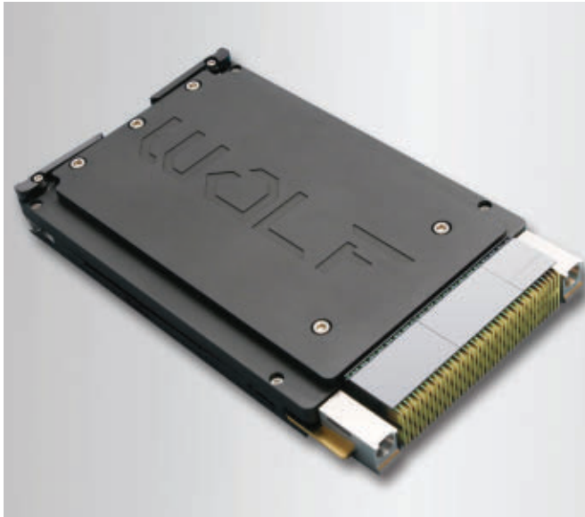
Curtiss-Wright's rugged VPX3-4925, VPX3-4935 (pictured above), and VPX6-4955 modules are designed to support compute-intensive ISR and EW systems.
